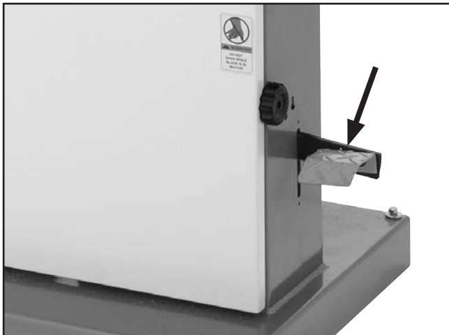
Figure 48. Foot brake location.
